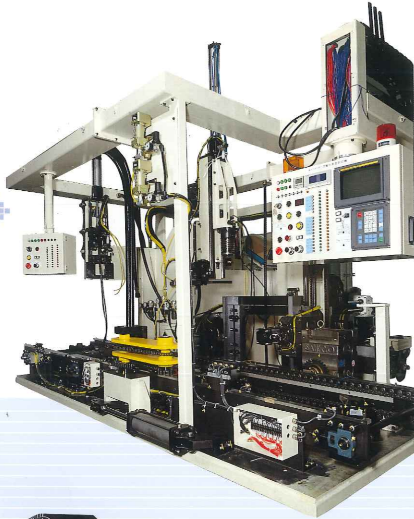
Measuring and marking machine for shaft bore of transmission case
